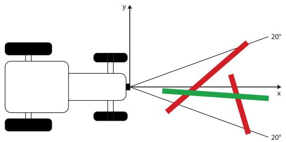
In the figure, the red lines are filtered. The green line is within the angle set to 20° and will not be filtered.
