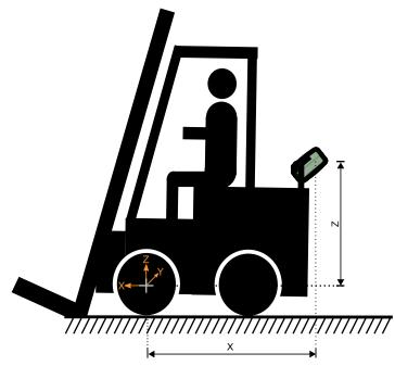
The reference point, the origin of the world coordinate system, is set in the front axle of the vehicle (grey cross). The distance of the device to the reference point on the X axis is entered in the field "X position of sensor". The distance of the device to the reference point on the Y axis is entered in the field "Y position of sensor". The distance of the device to the reference point on the Z axis is entered in the field "Z position of sensor".
