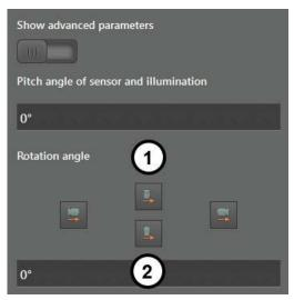
The angle of roll is determined and corrected automatically if the automatic calibration function is later used ( $\rightarrow$  "9.8 Automatic calibration").
