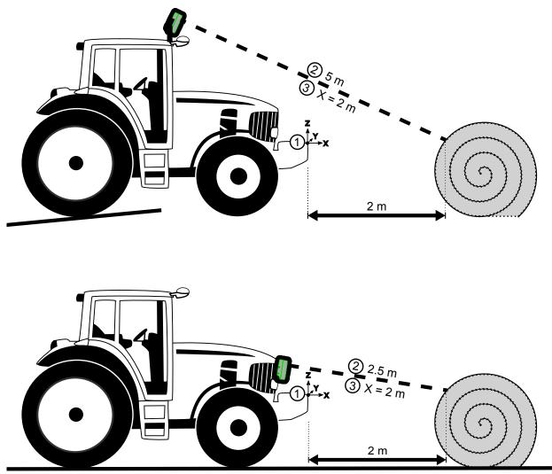
The image above shows two different mounting positions of the device on a mobile machine. In both cases, the world coordinate system is defined identically (1). For both mounting positions, the internal measured value of the device differs by the mounting position (2).
