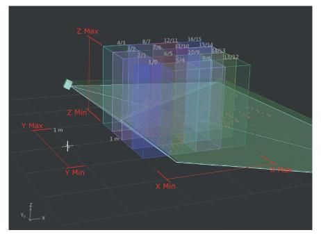
The "min/max values" for the x, y and z axis indicate the position of the grid in the world coordinate system. The three axes are marked in red in the figure above. The origin of the coordinate system is marked with a white cross. The grid of the level has a division of 1 m.
