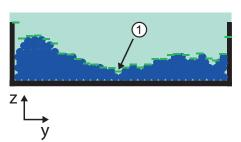
The figure on the left shows the result type "Min" with a 3D grid made of ROIs. The result is marked with ①.
