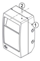
The reference point of the device is determined via the lateral reference socket (1). The reference socket cuts the coordinate origin in the middle of the sensor (2).
