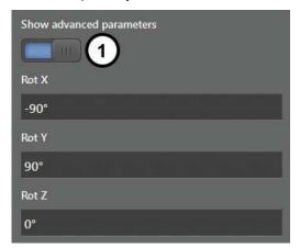
The image shows three input boxes for the rotation of the device. Depending on the orientation of the sensor, the input boxes already contain values ( $\rightarrow$  "9.4 Position of the device"). With the values, the overall rotation is calculated.
