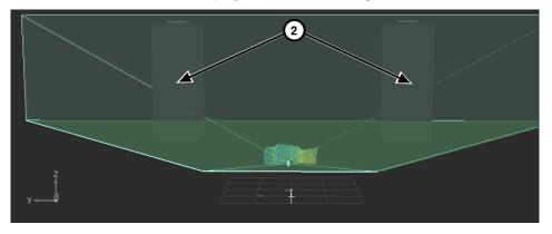
Set the exclusion area a bit larger than the objects to be excluded. Thereby, measuring errors on object edges caused by mixed pixels are excluded by further calculations.
