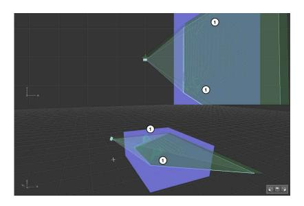
The markings (1) show objects in the search zone that interfere with the automatic calibration.
