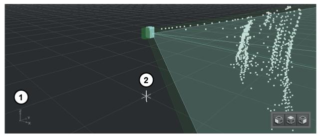
The world coordinate system is represented with its three axes (1). The coordinate origin is represented by a cross (2). The rectangular pattern on the X/Y level represents the ground level (grid 1 m). The Z axis looks up from the ground level. The X axis looks in the machine's direction of travel.
