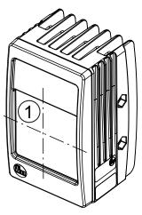
The reference point of the illumination unit is in the centre of the illumination screen (1).
