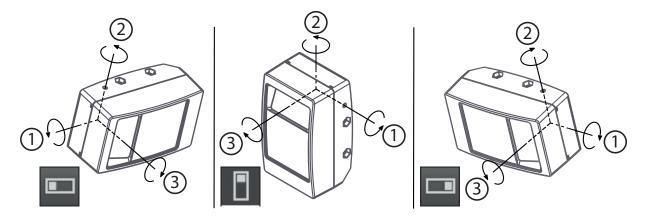
The figure shows the angles in relation to the orientation of the sensor.
