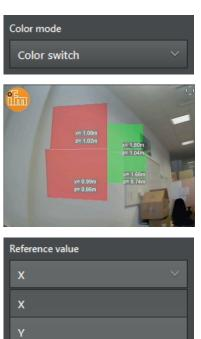
In the colour mode [Colour switch], there is a change between 2 colours when a threshold is reached.
