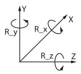
The overall rotation is calculated by multiplying the rotation matrices. The rotations around the X, Y and Z axis are described by the rotation matrices  $R_x$ ,  $R_y$  and  $R_z$ . The rotation matrices  $R_x$ ,  $R_y$  and  $R_z$  are formed internally from the Euler angles that are entered in the input boxes.
