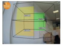
In the figure on the left, the output of 4 ROI groups is visualised as a coloured overlay and the X values as a text.
